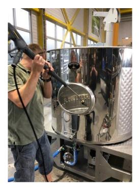
Best cleaning results can be achieved by a high pressure cleaner. On the Braumeister 1000 L it's possible to remove a manhole in front of the vessel for a better accessibility for cleaning, inspection and service.
