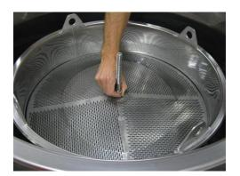
When the mashing-in temperature has been reached, a signal tone is emitted; press *Select* to acknowledge it. Then insert the malt pipe (with pulled-on seal facing downwards). Ensure that the seal is centred on the malt pipe and sits absolutely flush on the vessel base. Slide in the filter plate to the lower edge.
