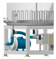
Start off by filling 230 L or 575L or 1200 L brewing water into the vessel (to the upper marking). The malt pipe is not yet inserted. The markings on the tie rod indicate the filling level of 170 L, 200 L and 230 L or 425 L, 500 L and 575 L or 700 L, 850 L, 1000 L, 1150 L, 1300 L. The valve position during the heating phase is shown in the illustration on the left-hand side.
