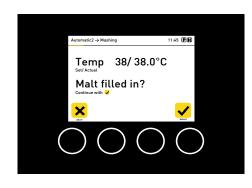
Once you have filled the malt, acknowledge it by pressing the *Select* button. For safety reasons, you will receive the prompt "Malt filled?" And by pressing *Select* the actual brew process commences with the Braumeister. The pump and the heating switch on. The wort rises up in the pipe and overflows. The cycle has begun and the malt is washed out by means of transfer pumping in the next phases.
