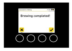
Once the boiling time has elapsed, another signal tone is emitted, indicating the end of the brewing procedure. Use the *Select* button to acknowledge it. The heating switches off.
