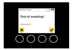
After completion of the programmed brewing phases, another signal tone is emitted. Press *Select* again to acknowledge it. The pump switches off and you are prompted to start purifying ("Remove malt pipe"). Purification means separating the crushed malt from the beer wort. Purifying with the Braumeister is a relatively easy, fast and clean exercise, compared to many other home brewing methods, and represents a central concept of the Braumeister. Remove the thumb screw including
