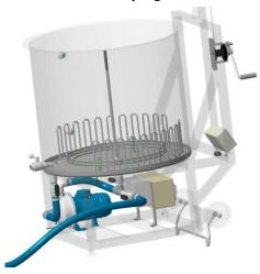
In order to position the Braumeister for cleaning purposes, fold down the rear bracket or turn the winch to tilt the Braumeister. Connect the hose to a drain pipe and position the valves as seen in the illustration on the left-hand side. Now, the Braumeister can be cleaned from the top, using an appropriate brush and water. The dirty water can be pumped (in 'Manual' mode) down the sewer drain.
